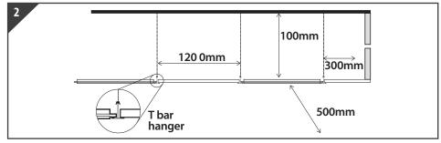
Ensure that there is adequate space for panel installation in suspended ceiling
