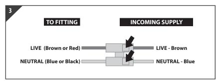
Insert correct supply and wiring from the driver into terminal block (not provided), tighten all screws in block
