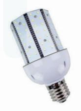
Heathfield LED Corn lamps are designed to replace the traditional sodium and metal halide products. This 30w version offer in excess of 4,000lm. The unique design of this lamp offers uniformed 360° light distribution, and an effective heat management system that incorporates an integral fan to maintain lumen stability. This lamp is a cost effective alternative to a complete fitting change, with a long lifespan and no maintenance costs this product is truly a fit and forget solution.
