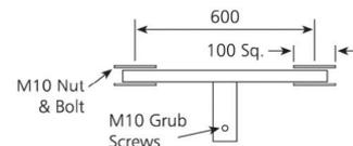
Most columns of 8 metres and above have a column spigot; we will ensure that the brackets ordered will fit your columns. Where brackets are purchased alone for existing columns please indicate the diameter of the column spigot.
